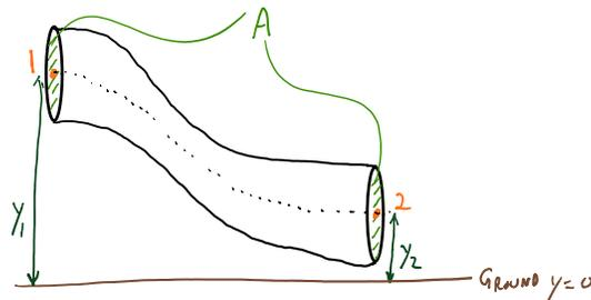
**PRACTICE:** Water flows from 1 to 2 in a pipe system like in the figure below. The cross-sectional area at point 1 is less than at point 2 and point 2 is higher in elevation than point 1. Which of the following statements are plausible. (drawing not to scale)
