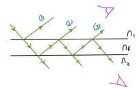
Multiple reflections and transmissions occur as seen above. The net effect does not change our mathematical model, eave adjacent wave (1 and 2, 2 and 3, 3 and 4...) maintain the same phase relationship as the first set (1 and 2) and the path length difference between each adjacent wave is still 2t (you should try confirming these statements). Showing more reflections does introduce an interesting idea; you can be on either side of the thin film to observe interference.
